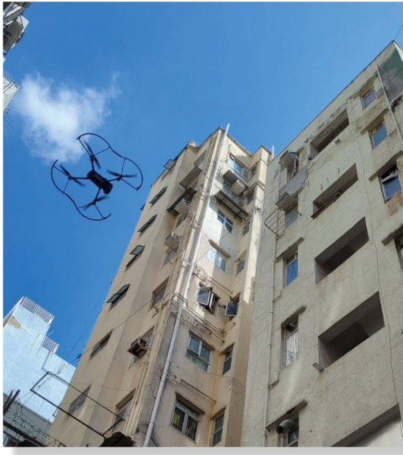
Figure 3: Survey of external walls of buildings conducted by BD using drones
